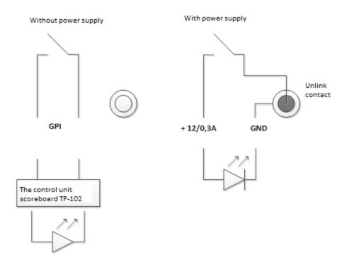
Without power supply to the "Red Light (Power)" power socket, the output for the light scoreboard works in GPO mode. The input connectors of the TR-141 "Control" unit A or B are connected to the output of the RCA-F console "Red Light (Out)".
