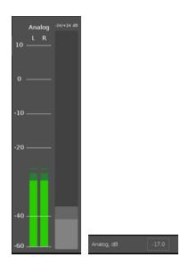
• using digital input. Touching the parameter value window on the display opens the digital input editor in which the required parameter value is entered. To apply the parameter, press **OK**.
