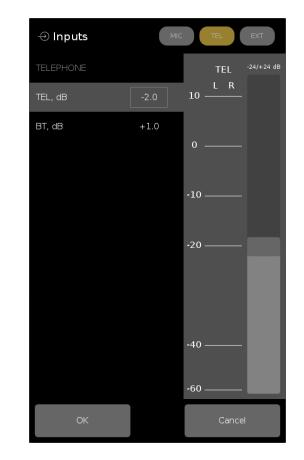
The input gain control is set to +/- 24 dB.
