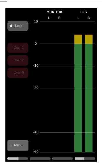
Lock - virtual button for blocking a rebroadcasting channel, the background color is gray. The Lock button becomes active only when the EXT button is red and turned on. The pressed Lock button turns green and locks the REC mode 1, 2, 3 and the state of channel 8. At the same time, the EXT button becomes bright green. Pressing Lock again deactivates the REC 1, 2, 3 and channel 8, the Lock button becomes gray again, and the EXT button turns red.
