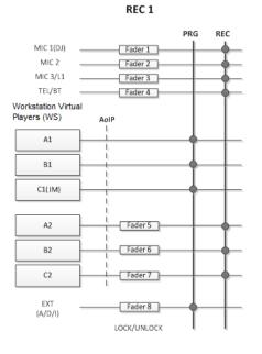
In a telephone conversation, the signal from MIC 1 (DJ) and TEL/BT channels go to the REC bus, and not to air.
