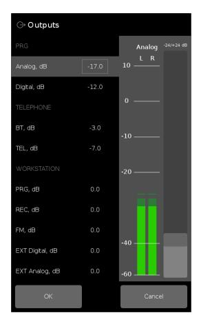
**PRG** are the main software outputs of **ANALOG** and **DIGITAL**. The adjustment range for each output is within +/- 24 dB relative to the level set for the program bus. The recommended level is + 4dBu (-20dBFS).
