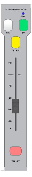
**Pair** - Blue LED indicates that two-way communication is established via **Bluetooth** between the external device and the mixing console.
