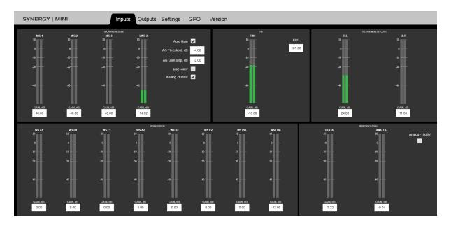
**AutoGain** allows you to turn on the system to automatically lower the microphone signal level.
