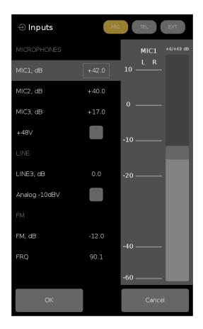
**MIC1, MIC2, MIC3 -** input gain lines for the three microphone inputs. Gain factors for input analog mic preamps are set using the digital value set in dB or the position of a virtual slider controller in dB. The adjustment limits are in the range of + 6 dB to + 69 dB with an adjustment step of 1 dB.
